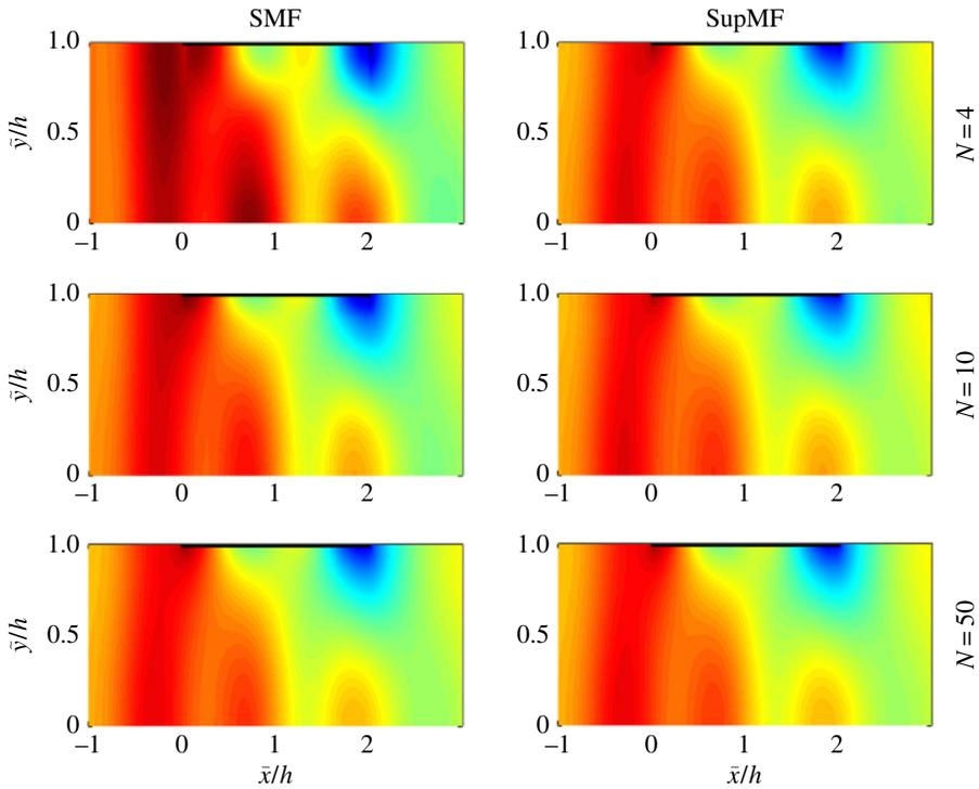
**Figure 2.** Wavefield (real part) in the waveguide, for  $M = 0.7$ , at frequency  $\tilde{k}h = 2$ , computed with the SMF (left panels) and SupMF (right panels) with  $N = 4, 10$  and  $50$ . The admittance is given by equations (4.1) with  $Y_1 = 1 - 5i$ ,  $\varepsilon/h = 0.1$  and  $\tilde{L}/h = 2$  (the part of the upper wall locally treated  $0 < \tilde{x}/h < 2$  is materialized by a thick black line).
