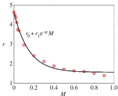
**Figure 4.** Variation of the convergence rate  $r$  with the Mach number in the SupMF formulation ( $\tilde{k}h = 2$ ,  $Y_1 = 5 - 5i$ ,  $\varepsilon/h = 0.1$  and  $\tilde{L}/h = 2$ ). Circles: values of  $r(M)$  calculated from the convergence curves (figure 3) with  $|R_\infty - R_N| \sim 1/N^r$ . Plain line: best fit of the data, with  $r = r_0 + r_1 e^{-\sigma M}$ , leading to  $r_0 = 1.5$ ,  $r_1 = 3.1$  and  $\sigma = 5.6$ . (Online version in colour.)
