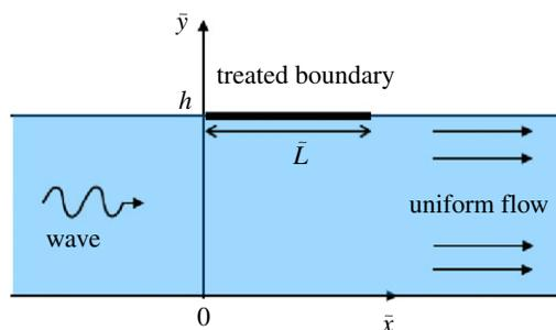
**Figure 1.** Waveguide with the upper wall characterized by a localized Myers boundary condition ( $0 \leq \tilde{x} \leq \tilde{L}$ ), Neumann boundary condition otherwise.
